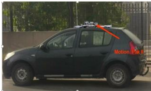
Figure 2. Motion pak II placement on the test vehicle
